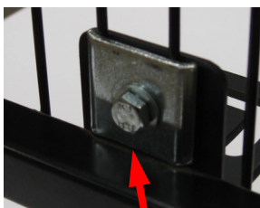
Square washer touching bottom of guard
